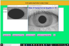
In above screen from uploaded image we extract IRIS features which is displaying in first image and then this image feeds to CNN and then CNN predicted that IRIS belong to person ID 15. Now I will upload one image from CASIA folder and then test whether CNN will predict correctly or not
