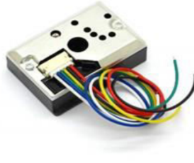
Fig .4: Dust Sensor.
