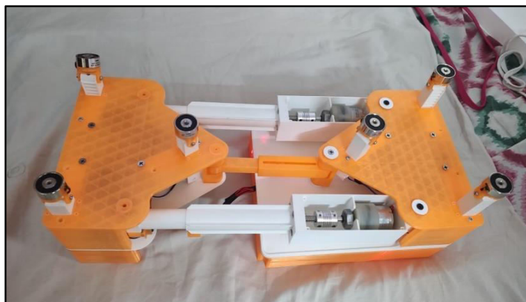
Fig 3.5: 3-D Printed Robot Model (Bottom View)
