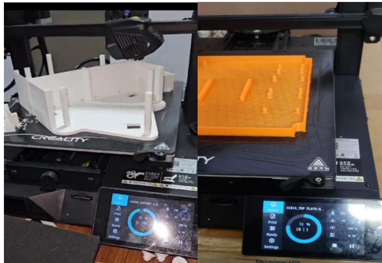
Fig 3.2: 3-D Printing of the TOP and BOTTOM Plates
