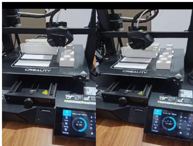
Fig 3.3: 3-D Printing of the side and Middle Links
