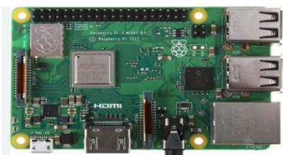
FIGURE 2: RASPBERRY PI 3B+
