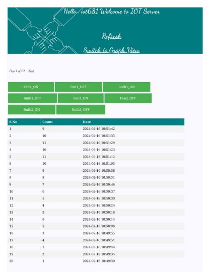
The entries of each and every person data is uploaded in the website by using ESP8266 IoT module. The entry and exit of the person is uploaded from time to time in the server and we can see and operate it at anytime from anywhere.
