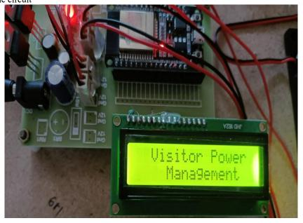
After providing power supply the title of the project will be displayed. The output is seen in the following image after we have connected the IoT module via a WIFI connection.
