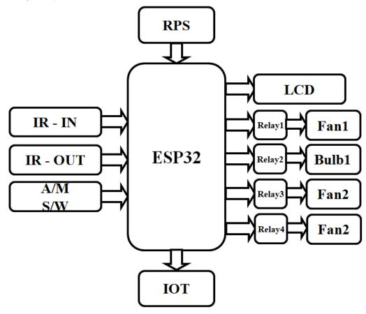
The above block diagram consists of IR-IN, and IR-OUT sensors which sense the persons entering and exiting the auditorium. And provided with two mode switches either automatic or manual mode, ON-OFF switch also given at input side.
