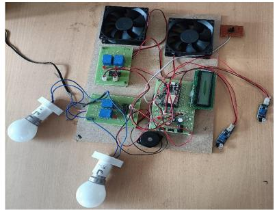
The above image shows the hardware equipment of the project. The kit is turned ON by giving the regulated power supply of 12v which is then converted to 5v dc current. The LED is the indication for 5v current so, if there is 5v current then automatically the LED glows. The generated 5v dc current passes to every hardware component in the circuit
