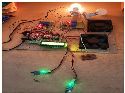
As shown in the above figure only one light and one fan is turned on as the count value is in the range between 1 to 10 members when it is in either automatic or manual mode.
