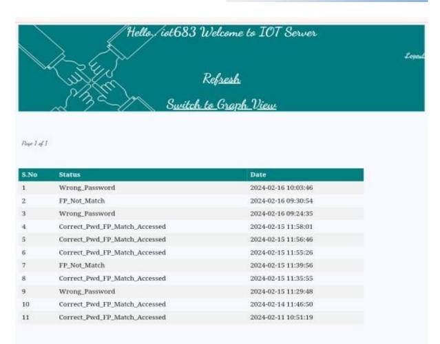
The entries of each and every person data is uploaded in the website by using ESP8266 IoTmodule.Here the authorized persons data and also if the unauthorized persons access the system then also the IoT module uploads data indicating wrong password, FP not match. This website is very useful to the owner of the bank locker to observe their system at any time and anywhere.
