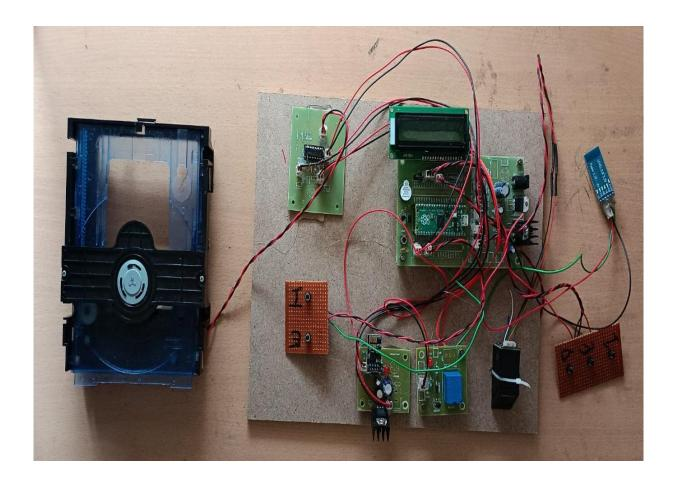
The above image shows the hardware equipment of the project. The kit is turned ON by giving the regulated power supply of 12v which is then converted to 5v dc current. The LED is the indication for 5v current so, if there is 5v current then automatically the LED glows. The generated 5v dc current
