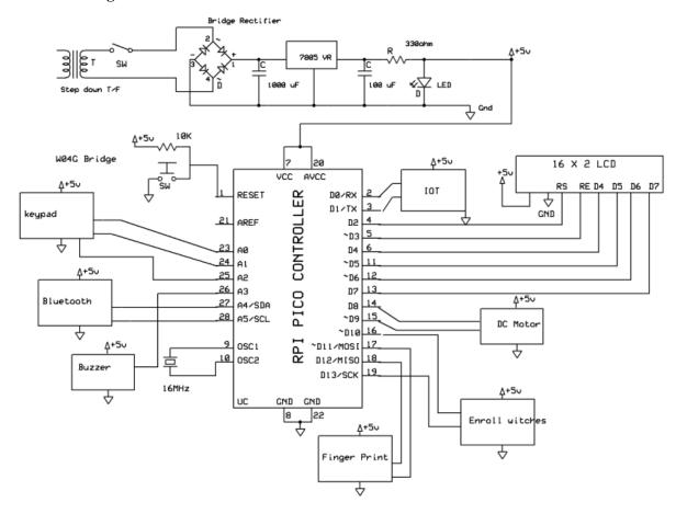
This is the pin diagram where all the hardware components are been connected components. this RPI PICO microcontroller having 28 pins. In which 14 GPIO pins as digital pins and 6 GPIO pins. 16MHz crystal oscillator connected internally. The step down transformer, Bridge rectifier capacitor with 1000f Resisters and led are connected in Regulated power supply which provide the 5v to the Arduino and all input/output modules.
