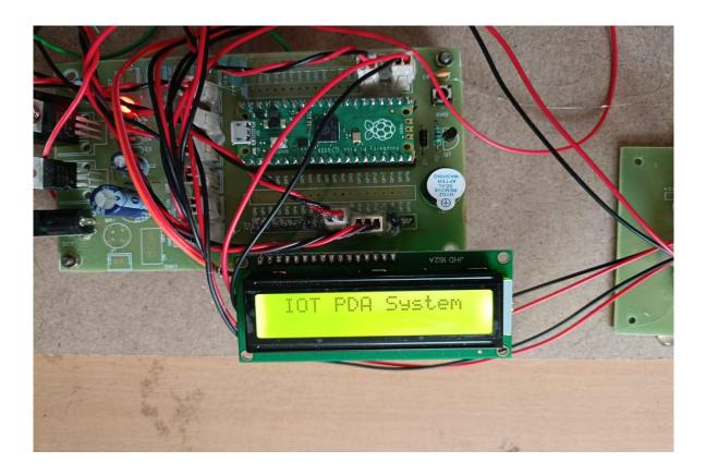
When we hit the reset button after providing the regulated power supply, the LCD displayed the IOT PDA System. The output is seen in the following image after we have connected the IOT module via a WIFI connect and after completing all the security verifications.
