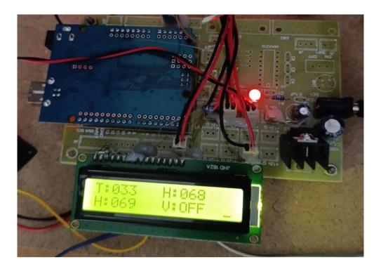
The System counting heartbeat and measuring body temperature correctly. Whenever beat count increase or decrease to certain level or body temperature increases or decreases below certain level system will display the current status of parameters. System also sends the exact location of the soldier when he or she press the panic mode switch to desired Registered Mobile Number through SMS .
