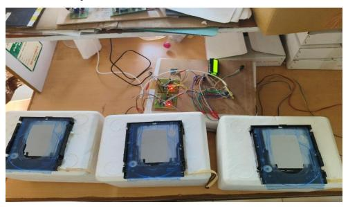
The pills are inserted in those boxes and boxes are opened according to RTC timings allotted in the IOT Android app .
