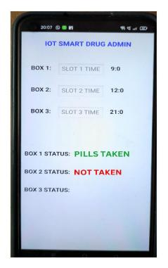
When the box is opened , the IR sensors are recorded that , pill is taken or not . The sensor detects human hand which we kept inside the box to collect our tablet. If the tablet is taken , by the server message is sent to IOT app that pill is taken in green color , if pill is not taken , it is displayed that no pill is taken from box in red color.
