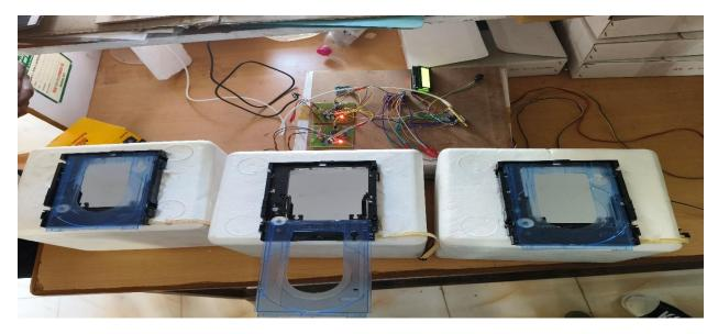
Above picture can be seen that how an box is opened to take the pills. The software coded so that the box will be closed within one minute automatically . When the box is open for every 10 seconds an buzzer sound will be coming from speaker upto the door closes .
