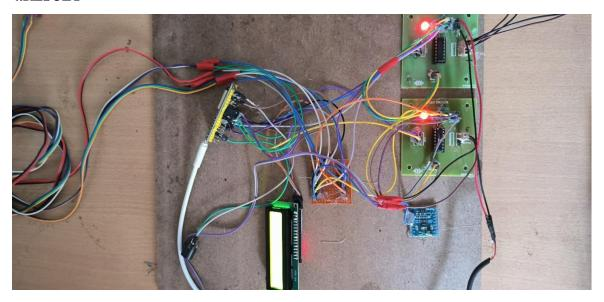
The above image shows the hardware equipment of the project. The kit is turned ON by giving the regulated power supply of 12v which is then converted to 5v dc current. The LED is the indication for 5v current so, if there is 5v current then automatically the LED glows. The generated 5v dc current passes to every hardware co component in the circuit.
