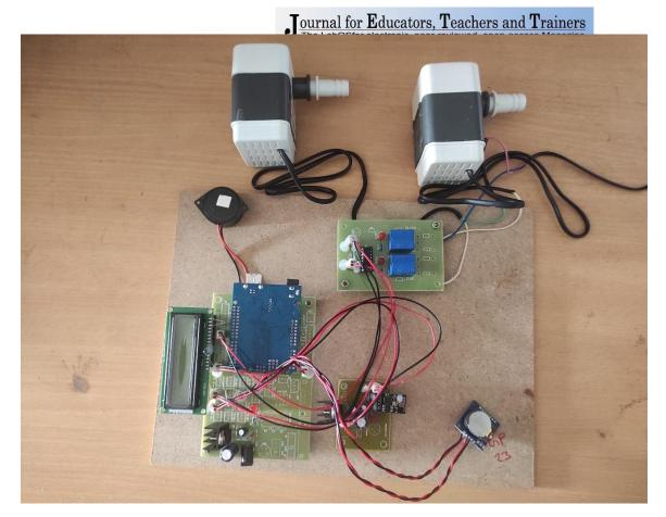
The above image shows the hardware equipment of the project. The kit is turned ON by giving the regulated power supply of 12v which is then converted to 5v dc current. The LED is the indication for 5v current so, if there is 5v current then automatically the LED glows. The generated 5v dc current
