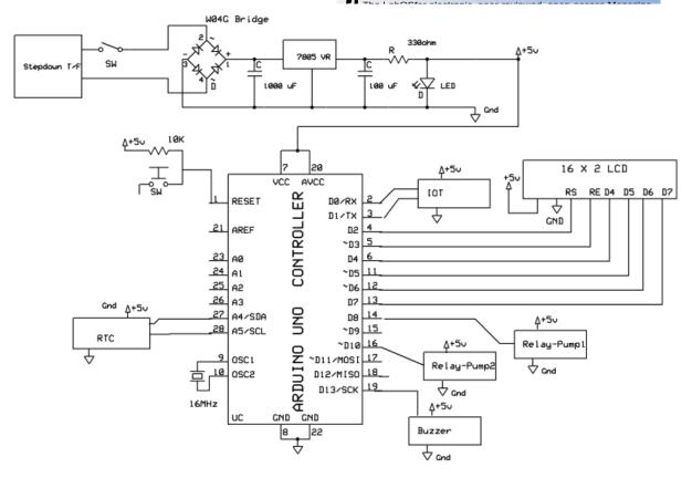
This is the pin diagram where all the hardware components are been connected components. this ARDUINO microcontroller having 28 pins. In which 14 GPIO pins as digital pins and 6 GPIO pins. 16MHz crystal oscillator connected internally. The step down transformer, Bridge rectifier capacitor with 1000f Resisters and led are connected in Regulated power supply which provide the 5v to the Arduino and all input/output modules.
