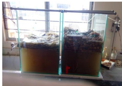
FIG 3.4: SEEDING (Sludge and wastewater ratio(1:1) for 15cm depth fibres)
